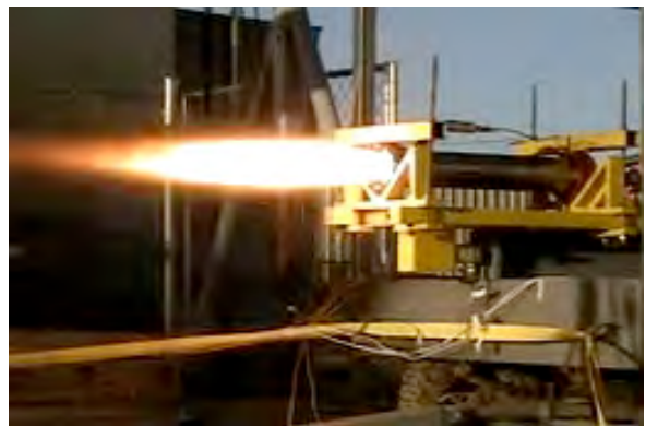
Project HALO TL-1 Flight Motor Static Test #3
